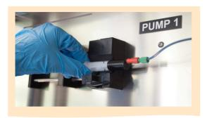
Steady flow rate is required to obtain high quality nanoparticles. Microstepping pumps allow precise flow rate control over a wide operation range. Syringes can be used as polymer reservoirs, allowing optimal flexibility and reducing time in changing polymer samples.
